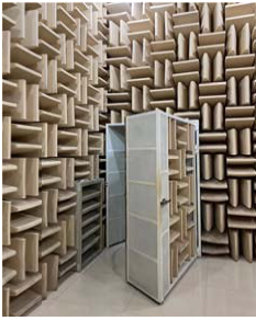
Semi anechoic room
